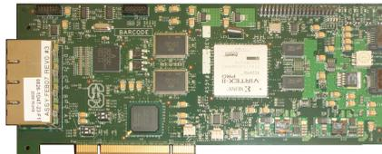
Figure C.3: Photograph of the NetFPGA circuit board
