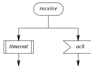
Figure B.3 – Inputs and Timeouts
